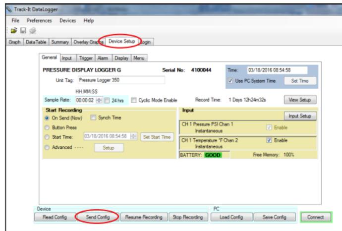
Review default factory configuration settings and make any necessary changes - sample rates, triggers, alarms etc. Be sure that the time and date is set properly.
