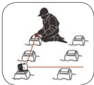
Level and square foundations with the LP4
